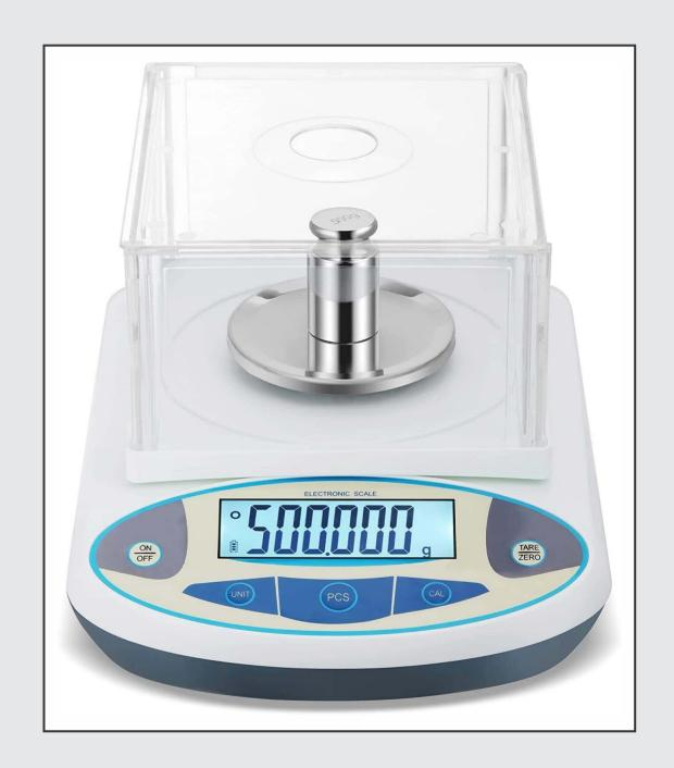
Calibration is the process of adjusting the set of scales so that its output is well calibrated.
